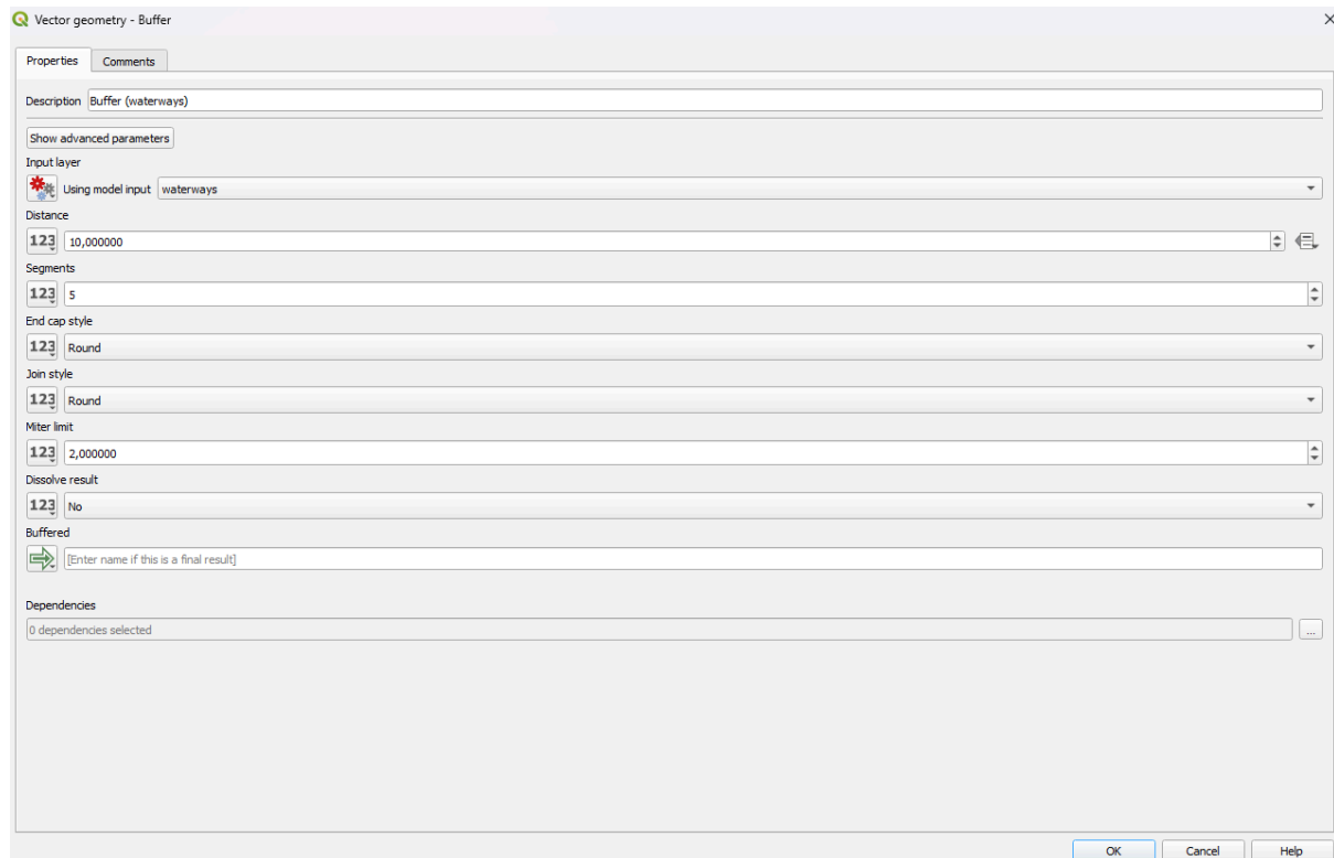
Image: Algorithm dialog of the buffer algorithm
